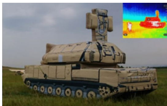
Figure 2: Decoys with Advanced Thermal Signatures
