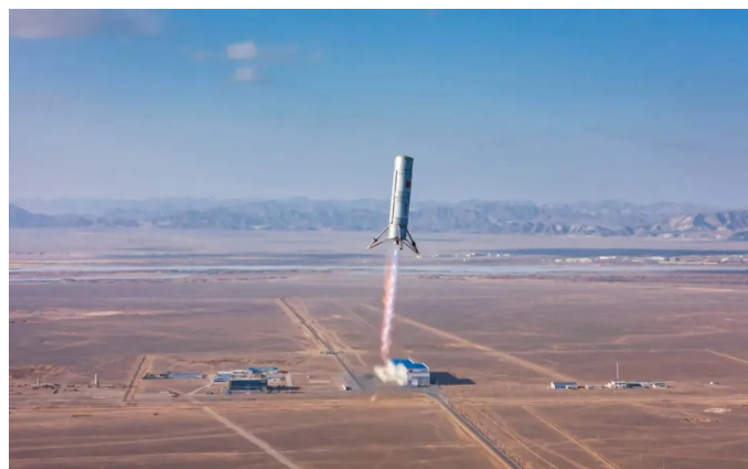
Landspace's Zhuque-3 VTVL-1 test article during a first hop test, Jan. 19, 2024. Credit: Landspace
