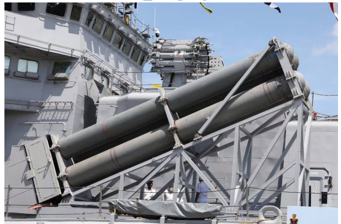
A quad launcher for BrahMos supersonic cruise missiles is seen mounted aboard the Indian Navy's guided-missile destroyer INS Delhi. (Gordon Arthur/Staff)
