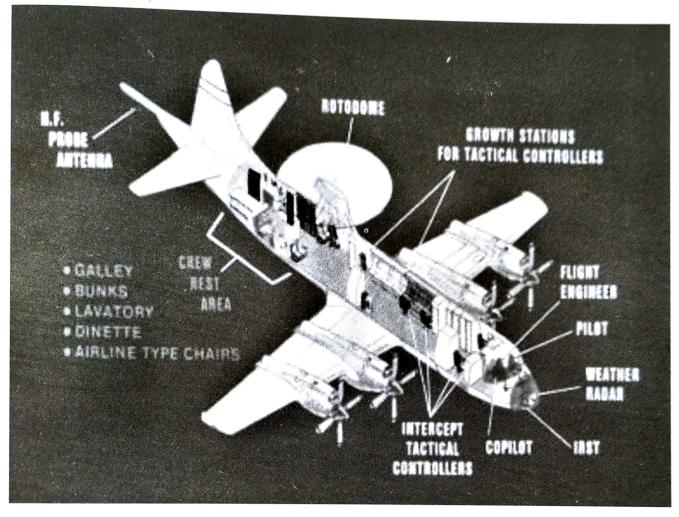
The Hawkeye's UHF radar has been integrated with both the Lockheed P-3 and C-130 airframes, providing a mid-range system with substantially better range and endurance performance than the E-2C. These derivative systems exploit the additional airframe volume available and use larger and newer computer and display technology, in comparison with the cramped E-2C airframe. Downloaded from www.ausairpower.net/aew-aesa.html on 23 Jan 2007
