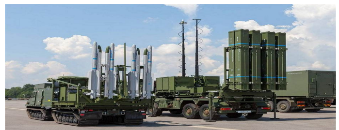
The launcher weapon station of the Iris-T missile can be mounted on tracked or wheeled chassis. (Picture source Diehl Defense)
