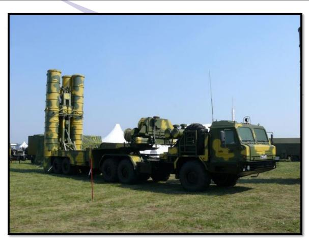
Image: S-400 Triumf (SA-21) Surface to Air Missile in vertical launch position with its TEL vehicle (Transporter Erector Launcher). Photo Source: Army Recognition
