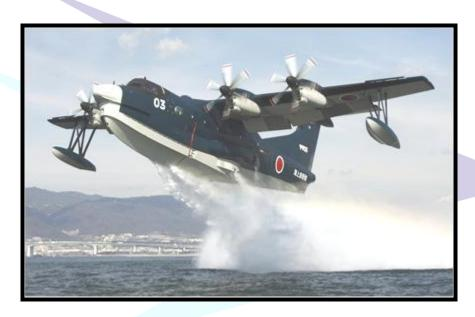
US-2 is an amphibious short take-off and landing (STOL) aircraft manufactured by Japan-based ShinMaywa Industries. Designed for air-sea rescue missions, the US-2 is operated by the 31st Fleet Air Wing of the Japan Maritime Self-Defence Force (JMSDF)<sup>i</sup>.
