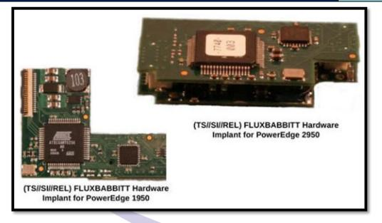
For GODSURGE to conduct its task, the target system has to be rightly fitted with JTAG scan chain and the hardware implant FLUXBABBIT through interdiction. FLUXBABBIT has to be pre-programmed with GODSURGE application code, the payload and the implant installer. Once the target system powers on GODSURE will occur and its frequency of execution is configurable. The cost of FLUXBABBIT hardware implant and to install GODSURGE in it is together estimated to be \$500.<sup>3</sup>
