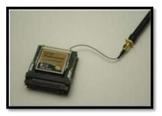
Mini PCI slots for added functions like GPS and multiple Wireless Network Interface Cards. This tool collects the WLAN networks from the specified location and maps them. This tool also gives the option for connecting more PCI devices to it for the purpose of wireless command and control or to install second or third 802.11 card. The unit price of this tool is \$6K.<sup>3</sup>
