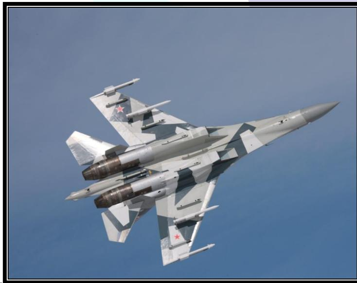
*SU-35 showing its hard points. Each wing has four hard points – one on the wingtip and three under-wing stations. There are two hard points on the underside of the fuselage on the centreline and one under each engine. Photo: Sukhoi Company website*
