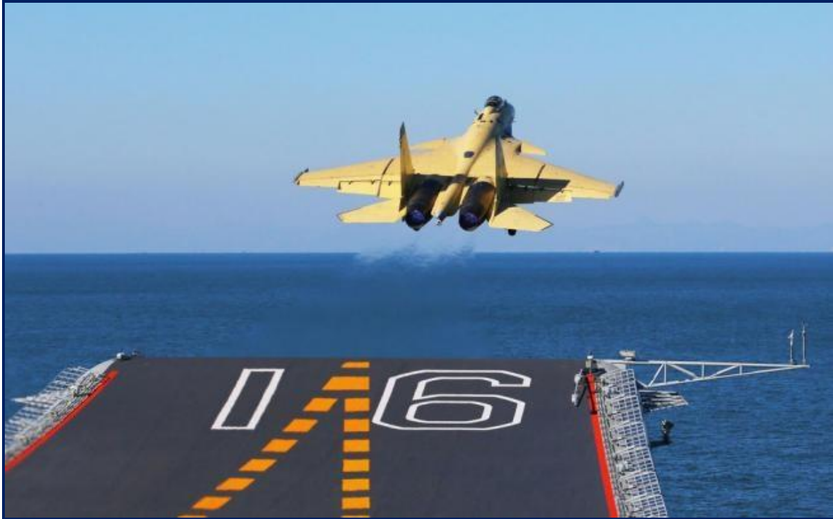
A J-15 fighter taking off from Liaoning aircraft carrier's Ski Jump Flight Deck
